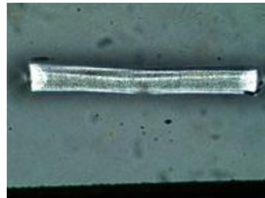
Fig. 1 Left: Output power vs. pump power obtained from a YAG/Yb:YAG ceramic waveguide. Right: picture of the waveguide input (the area shown in the picture is 2.42 x 1.82 mm)
