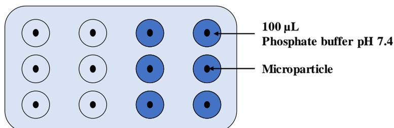
**Figure 1. Schematic presentation of the experimental set-up used for drug release measurements from *single* microparticles.**
