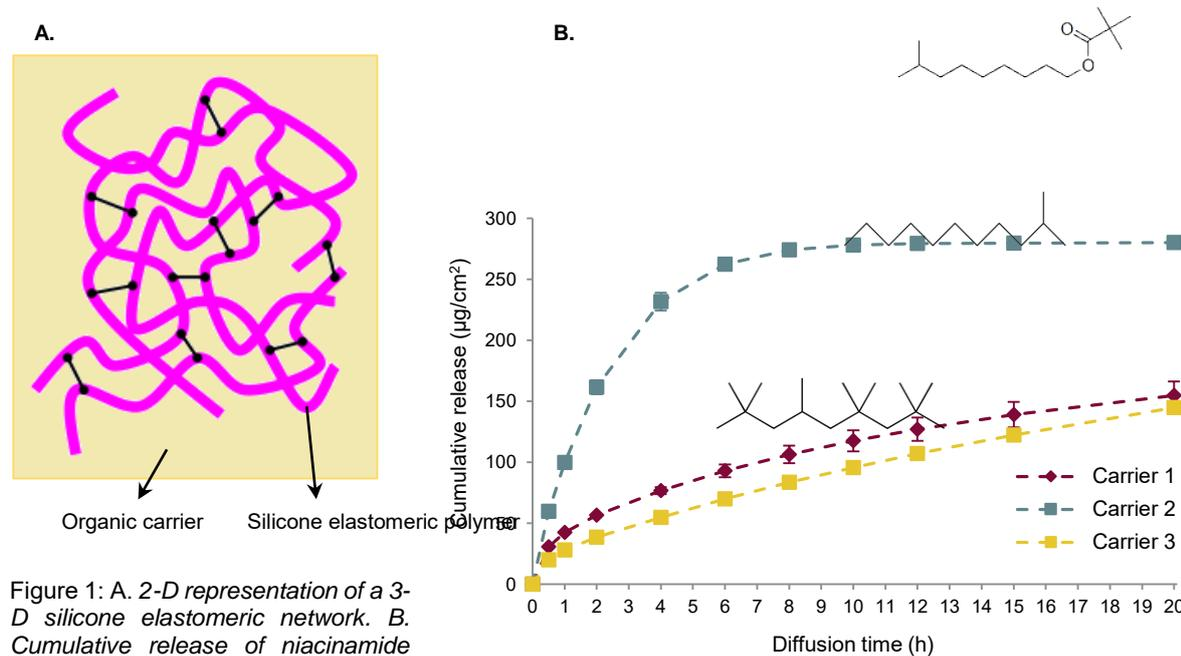
Figure 1: A. 2-D representation of a 3-D silicone elastomeric network. B. Cumulative release of niacinamide formulated into three water-in-silicone systems varying by the nature of the organic carrier used to disperse a silicone elastomeric polymer.
