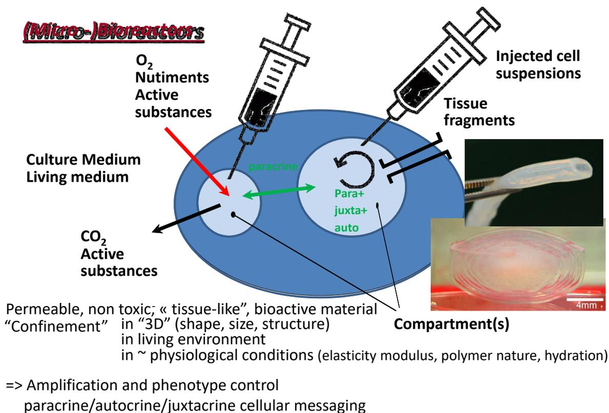
**Figure 1.** General scheme of the compartmented micro-bioreactors. Cells of different types can be inserted in the different compartments (Ladet 2011). The hosting system must preserve the diffusion of metabolites, oxygen, nutrients and the biomolecules implied in autocrine, juxtacrine, paracrine and cell messaging's. Such signalling is hypothesized to be enhanced due to a 'confinement effect' within bioreactors leading to specific maturation or differentiation effects.
